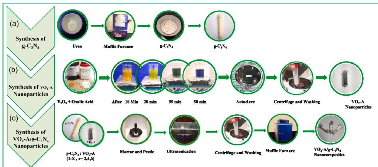
Scheme 1. Synthesis route of \text{VO}_2\text{-A/g-C}_3\text{N}_4 nanocomposites
